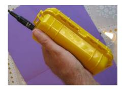
2) The second unit is provided by BigRedBee (<u>www.bigredbee.com</u>) and provides 5W of transmitting power using only 6-AA batteries. It is slightly smaller and therefore easier to pack. However, it has less transmitting power than the Byonics unit.
