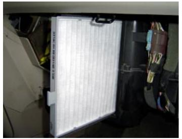
Install new filter, making note of air flow arrows. The air flow is from right to left. Install filter cover, making sure that it snaps into place.
