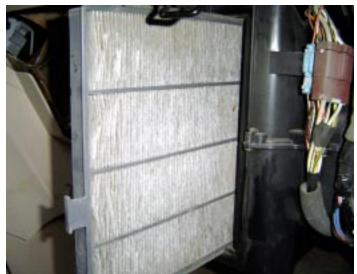
Use vacuum cleaner to vacuum area where filter was removed. A small nozzle placed inside heater unit will aid in removing debris that escaped the filter unit. Care must be taken not to damage any internal parts within the heater unit.
