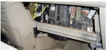
The next step is to remove plastic support. This support is used in the factory to help keep unit rigid for assembly. Removal of support will not affect structural rigidity. To aid in removal of plastic support, remove two lower dash attaching screws. This allows the bottom of dash assembly to be more flexible.
