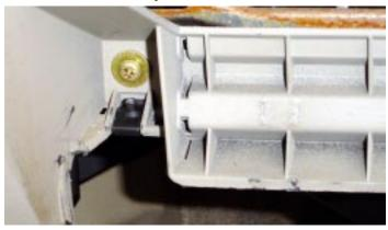
Using a sharp utility knife, cut plastic support downward at the notched area on support. I used a knife with replaceable blades, as a sharp blade makes the cutting much easier.
