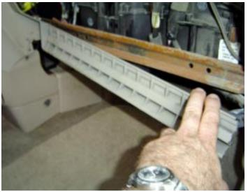
Once the plastic support is cut at both ends, remove support and discard.
