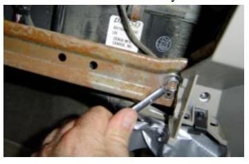
With bracket removed you now have access to cabin filter retaining cover. To remove this cover, grab cover at bottom of cover and pull down and out. This cover will pull out from the bottom and un-hook at the top. You now have access to filter.
