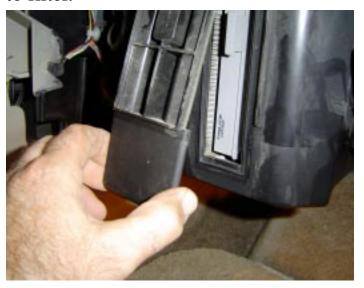
Grab filter by the small handle and pull straight out toward the rear of van. Note colour of filter compared to new filter.
