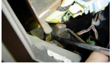
Remove right hand bolt from bracket and remove bracket assembly.
